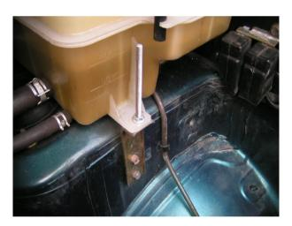
Remove the bolt from the header tank and replace with the short length of steel rod and nut as shown. The long length of rod can now be fitted to the threaded hole in the battery tray and locked in place with a nut and washer.
