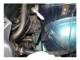
Lower the battery tray into position and check alignment of all mounting holes, the battery tray support can be adjusted slightly if required, and fix using four bolts and washers.
