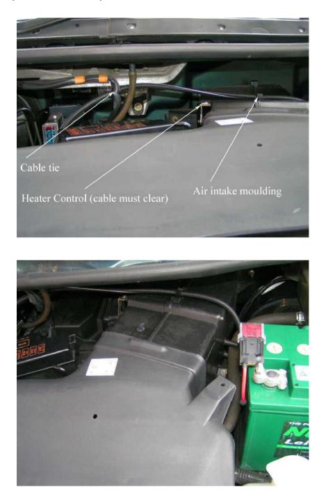
The earth lead for the Leisure battery should now be fitted. The leisure battery feeds are now live; you may confirm this by testing the interior lights and power sockets.
