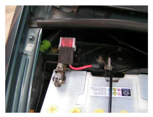
The leisure battery can now be fitted into its tray but **DO NOT FIT THE EARTH LEAD TO THE LEISURE BATTERY AT THIS STAGE!** But leave it tucked out of the way.
