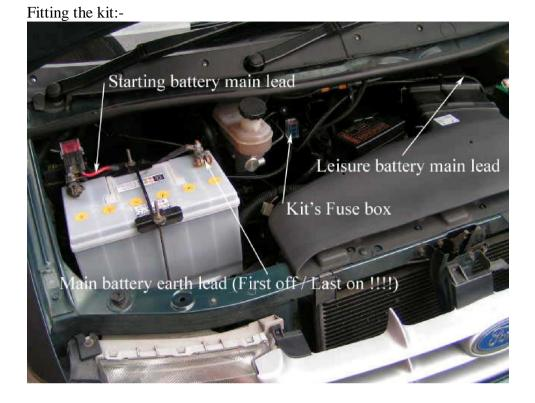
Remove the negative (earth) battery terminal from the main (starting) battery (make sure it's tucked down the side of the battery out of the way).
