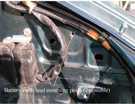
The main part of the kit can now be fitted. Start by passing the bundle of cables through the hole in the bulkhead from where the blanking plate was removed and fit the new plate with the nuts and washers provided. (It is recommended that a small area of paint is removed from inside the vehicle, around the holes in the bodywork, before fitting the two nuts and washers as this will insure a good earth for the kit)
