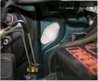
The foam seal on the rear of the blank can be carefully removed and fitted to the mounting bracket of the kit.
